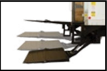
Standard Ramping Ride Gradual tilt throughout ride
