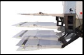
GLR- Gentle Level Ride™ Level ride with ground level tilt
