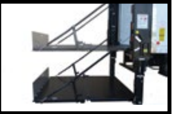
Full Level Ride Remains level throughout the cycle
